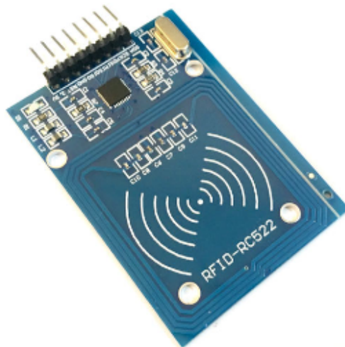
Figure 25: RC522 RFID Module
