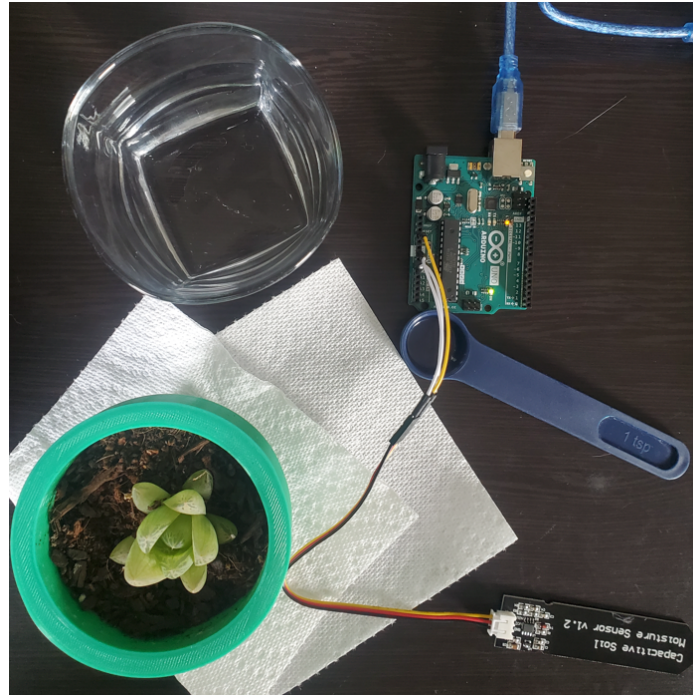
Figure 41: Soil Moisture Sensor Testing
