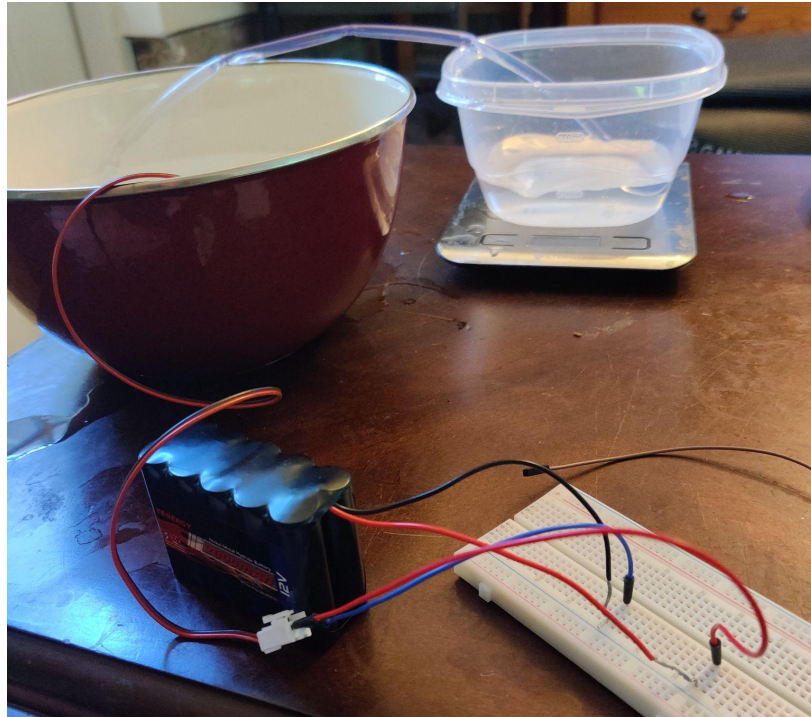
Figure 39: Pump Testing Configuration
