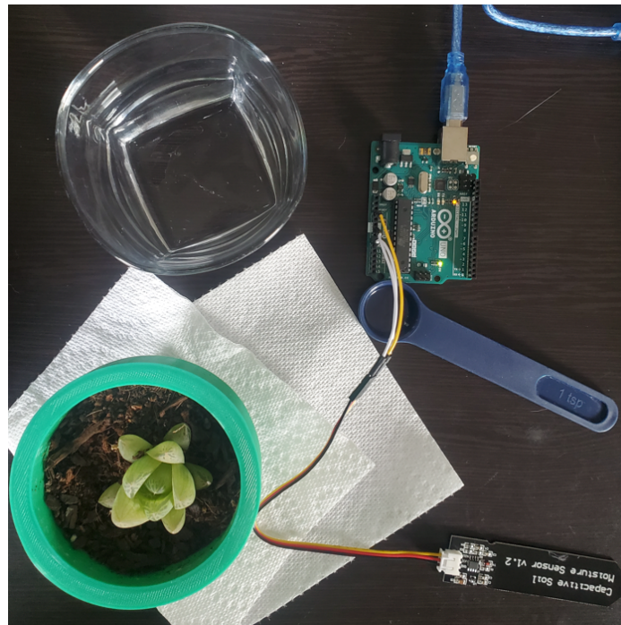
Figure 38: Soil Moisture Sensor Testing
