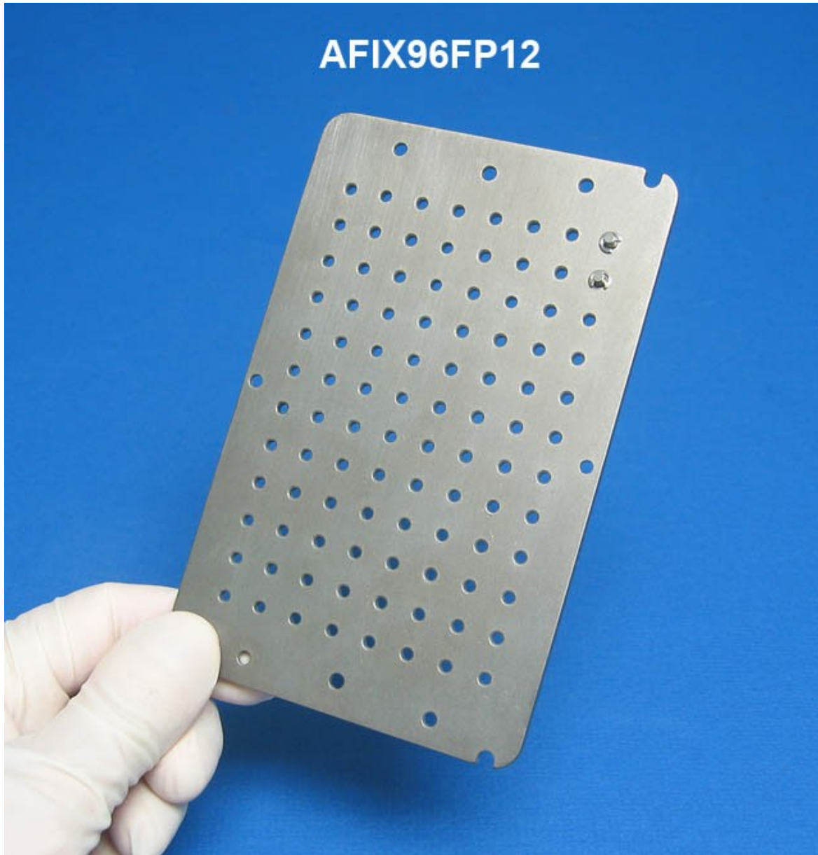
Figure 34. An example 96 pin fixture. Basic Robot Pin Tool Fixture for 96 FP12 Pins, single float plate, 2.36mm diameter pins, fixture plus spacers. Courtesy V&P Scientific.
