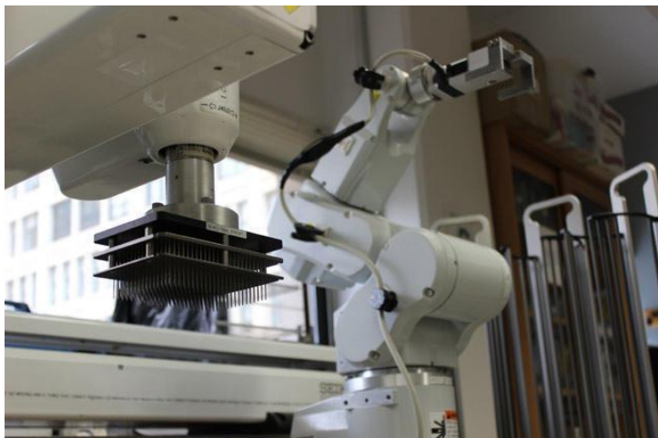
Figure 32 - Seiko Compound Transfer Robot (reprinted with permission from ICCB-Longwood Screening Facility at Harvard Medical School, Boston MA)
