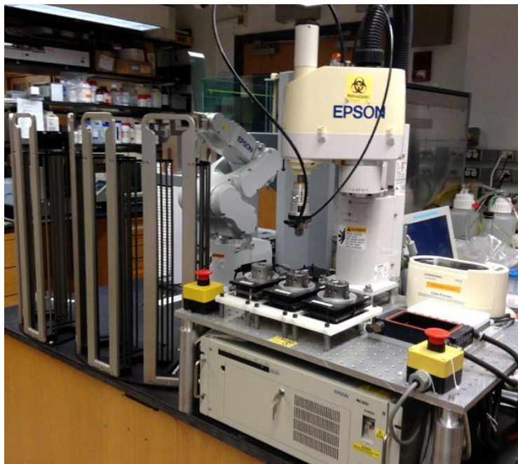
Figure 31 - Epson Compound Transfer Robot (reprinted with permission from ICCB-Longwood Screening Facility at Harvard Medical School, Boston MA)
