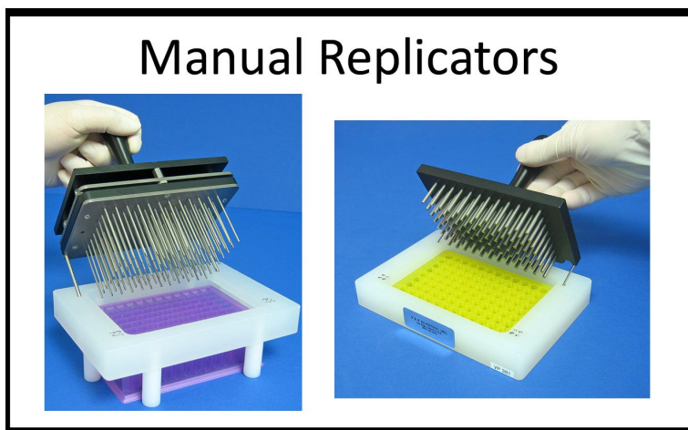
Figure 35. Manual pin transfer tool with key plate to ensure proper insertion. Courtesy of V&P Scientific
