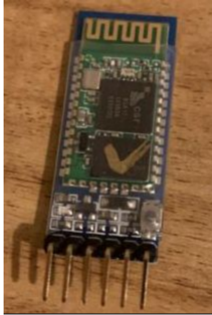
Figure 44: HC-05 Bluetooth 2.0 Module
