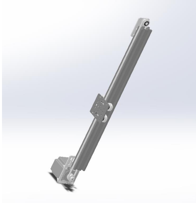
Figure 4. Linear belt driven actuator Solid Works CAD model
