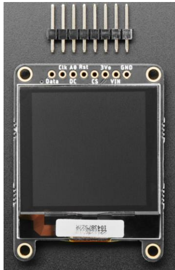
Figure 46 - Grayscale 1.5" OLED display (permission from Adafruit)
