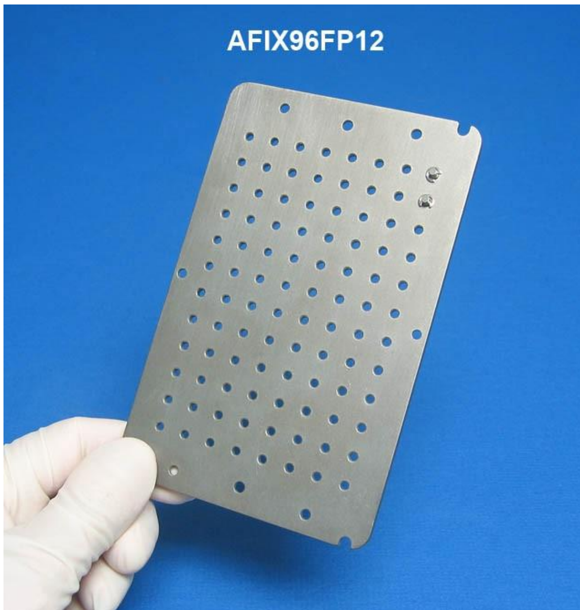
Figure 27. An example 96 pin fixture. Basic Robot Pin Tool Fixture for 96 FP12 Pins, single float plate, 2.36mm diameter pins, fixture plus spacers. Courtesy V&P Scientific.
