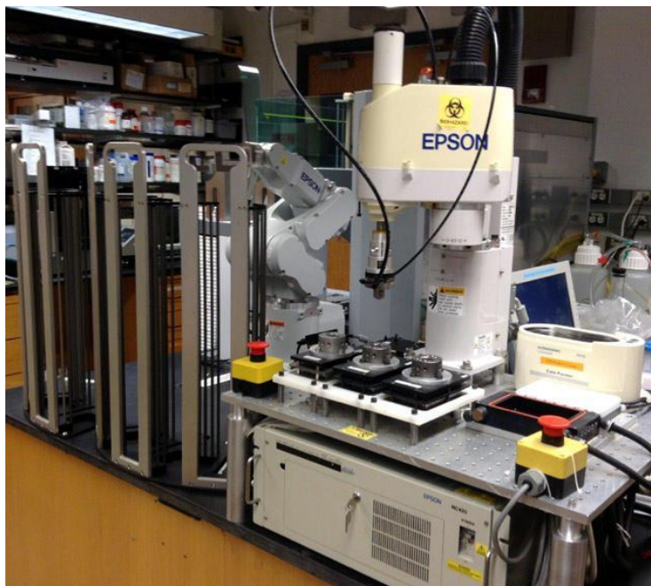
Figure 24 - Epson Compound Transfer Robot (reprinted with permission from ICCB-Longwood Screening Facility at Harvard Medical School, Boston MA)
