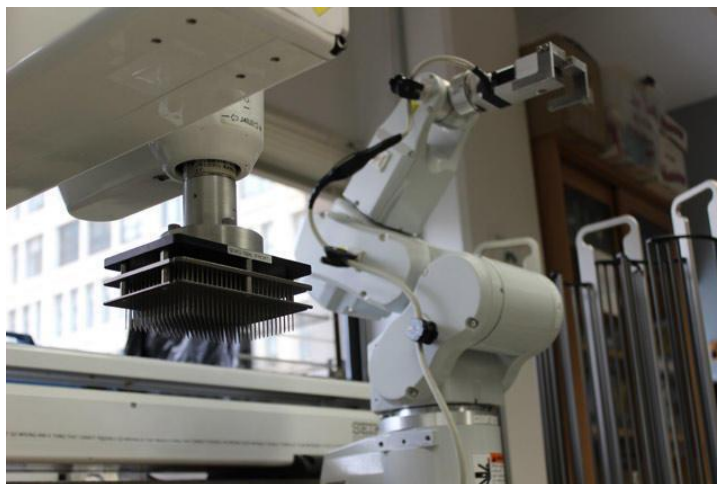
Figure 25 - Seiko Compound Transfer Robot (reprinted with permission from ICCB-Longwood Screening Facility at Harvard Medical School, Boston MA)
