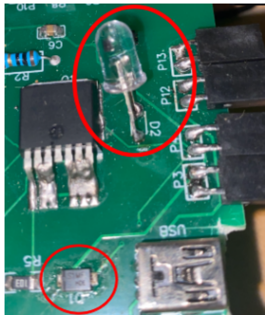
Figure 53. Weight Sensor SMT Diode Replaced with LED
