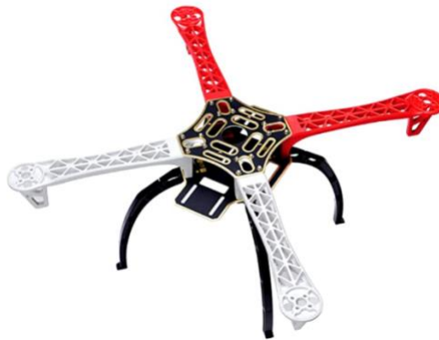
Figure 43: Drone Frame of Project
