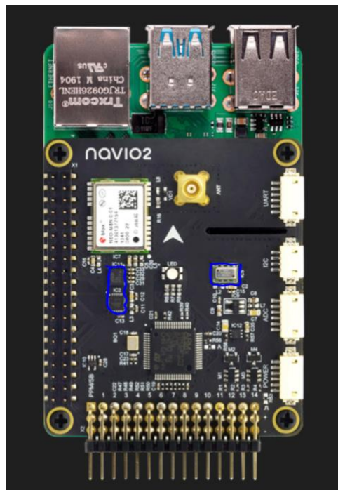
Figure 50: Blue Circled Sensor Packages on Navio 2
