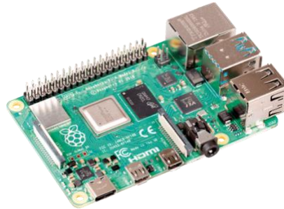
Figure 49: Data Processing Board Raspberry Pi 4b
