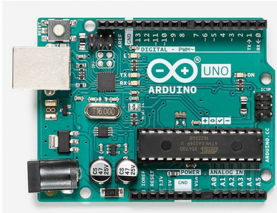
Figure 3.33 Arduino Uno Overview
