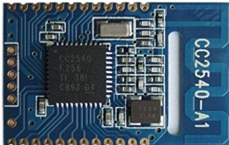
Figure 3.30 RioRand Bluetooth Chip Overview
