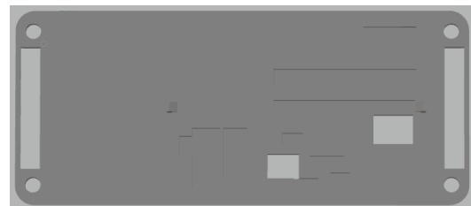
Fig. 15. View of the inside of the bottom of the casing. It has ridges to allow for the components to sit comfortably on the inside.
