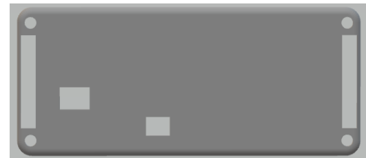
Fig. 14. View of the bottom part of the system casing. Shown are the holes for the pulse oximeter and sensitive parts of the PCB that cannot be closed off.
