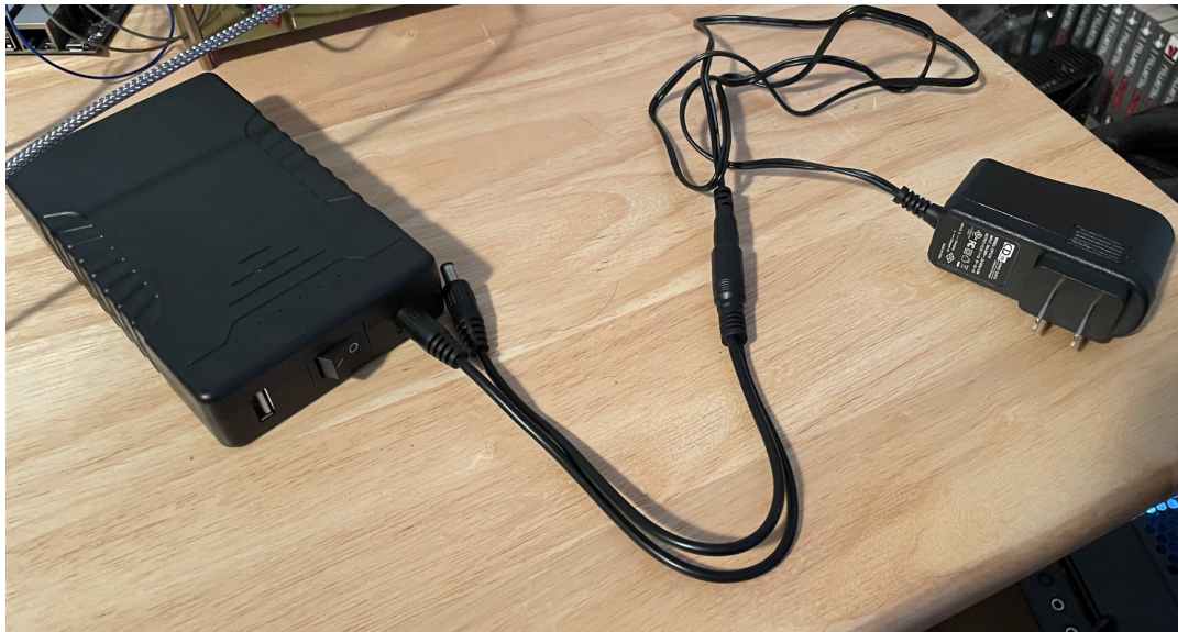
Figure 45 (Battery): Our 66.6 Wh battery and its coord/wall adapter. We soldered the split cable and it allows the device to power off of the wall while charging the battery.
