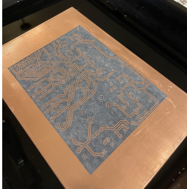
Figure 42 (Toner and Copper Plate Step Pt. 2): After rubbing off most of the paper.
