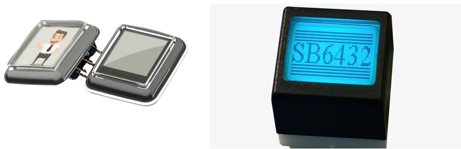
Figure 58 (Sample Segmented Options): Two pictures to help depict how the separated displays might look. The left is the aforementioned SuzoHapp product. On the right is one produced by LCD-Keys (I/O Universal Technologies).
