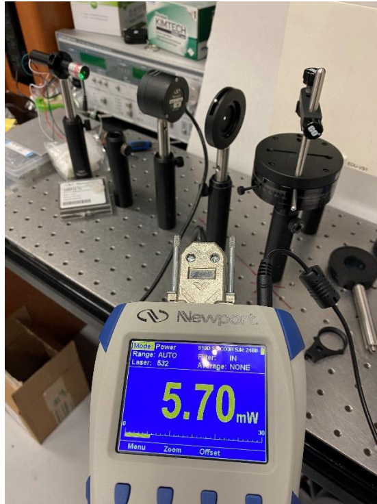
Figure 34. Output Power of 532 nm Laser Diode Module.
