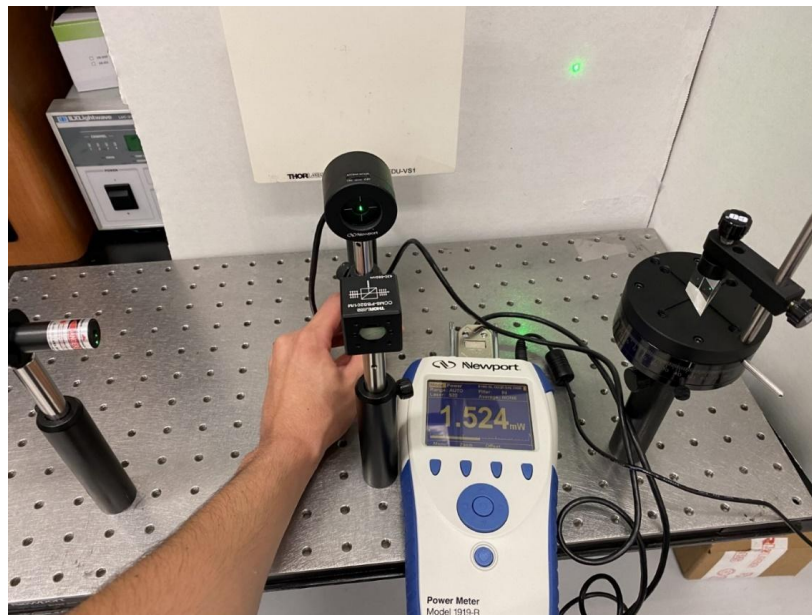
Figure 48. Measured Output Power of S-Polarized Light.
