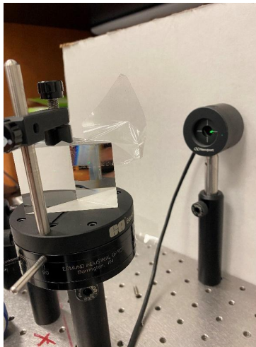
Figure 44. SPR Chip Attached to 40 mm Right-Angle Prism.
