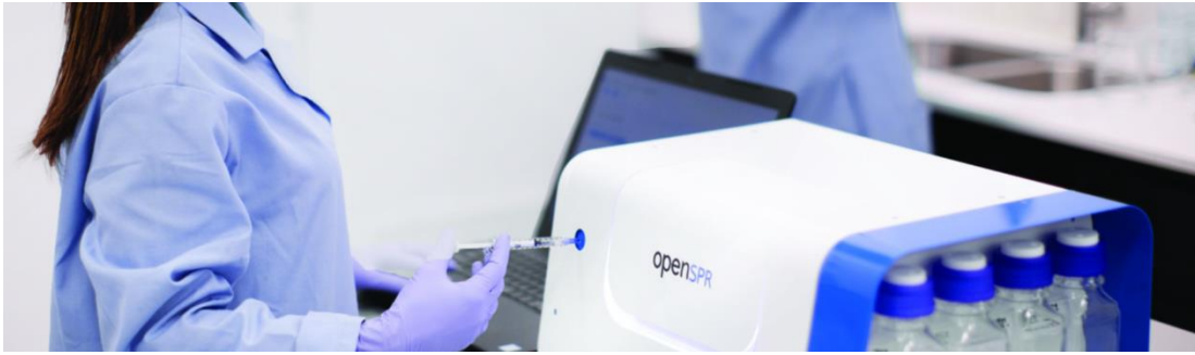
Figure 1. OpenSPR Surface Plasmon Resonance Sensor by Nicoya [approval for image from Nicoya pending]
