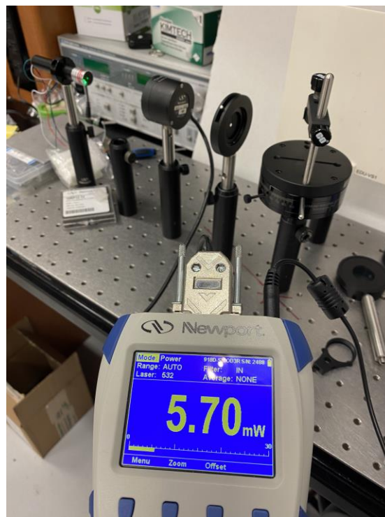
Figure 34. Output Power of Laser Diode from Edmund Optics
