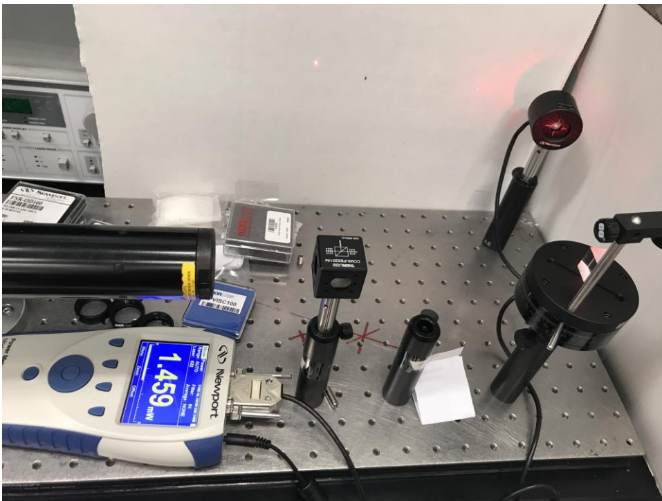
Figure 39. Experimental set up that displays an angle beyond the total internal reflection angle that results in power loss.
