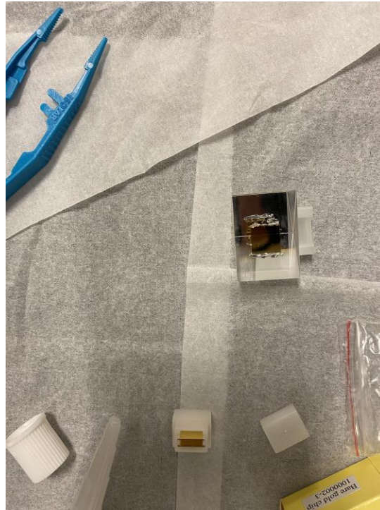
Figure 41. Attaching the SPR chip to the Right-Angle Prism.
