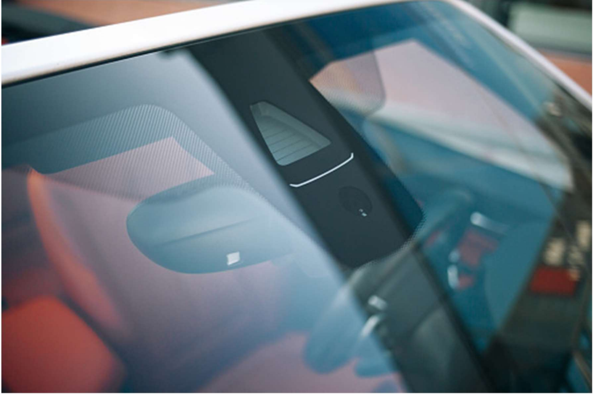
Figure 3.5.4.1: An example of a light sensor for an automobile, located behind the rearview mirror and against the windshield.
