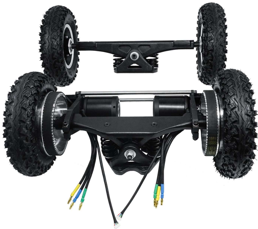
Figure 3.3.1.1.1: Wheels powered by belt motors
