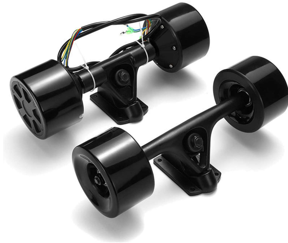
Figure 3.3.1.2.1: Wheels powered by hub motors
