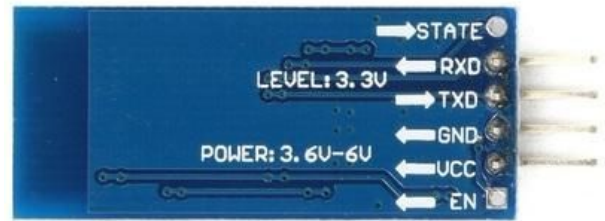
Figure 2: Bluetooth module HC-05 pinout.
