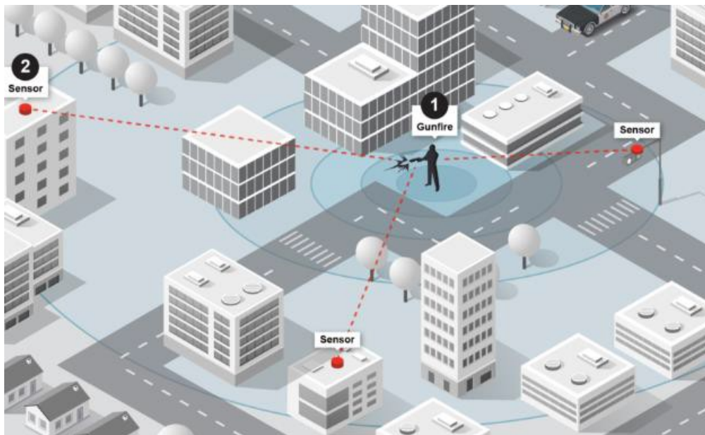
Figure 3-3: Example of how the ShotSpotter technology works.
