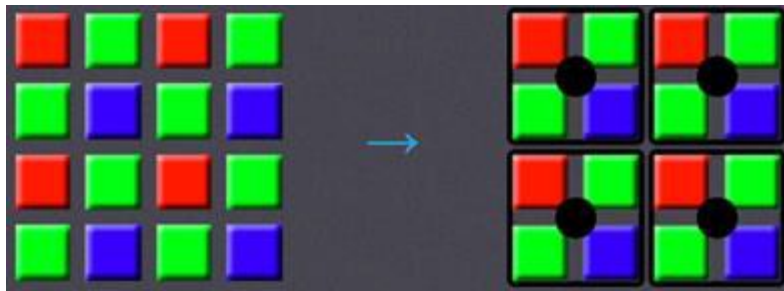
Figure 3-6: Bayer Array [“Digital Camera Sensors”]
