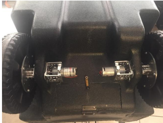
Figure 56: Assembled Motor Housing & Wheels
