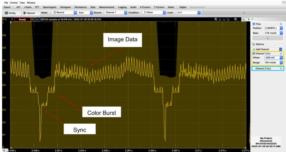
Figure 7.9: Camera Video Signal Test Result
