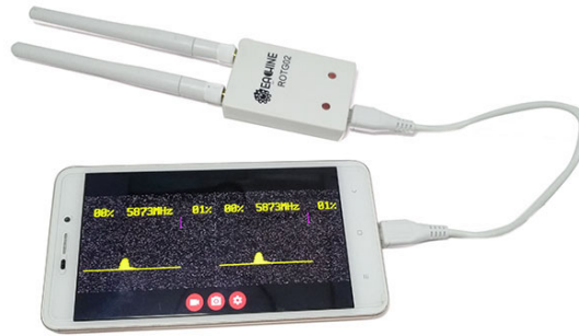
Figure 5.20: Example of the Video Receiver and Phone Connection (Permission Requested to Reproduce)
