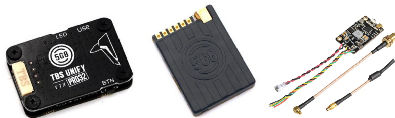
Figure 3.36: TBS Unify Pro32, TBS Unify Pro 5G8, and Eachine TX805 (left to right) (Permission Requested to Reproduce)
