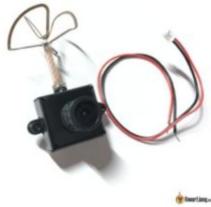
Figure 3.20: Camera with Built-in Transmitter (Permission Granted to Reproduce)
