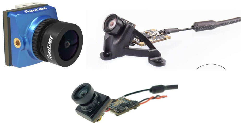
Figure 3.33: RunCam Phoenix 2 (top left), BETAFPV Z02 (top right), and Caddx Firefly (bottom) (Permission Requested to Reproduce)
