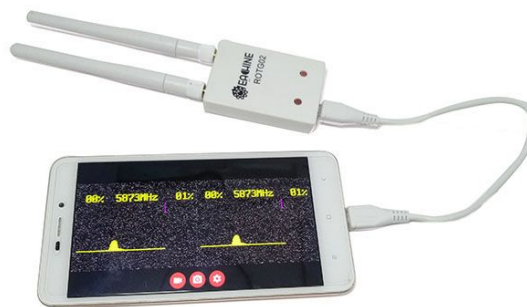
Figure 5.19: Example of the Video Receiver and Phone Connection (Permission Requested to Reproduce)
