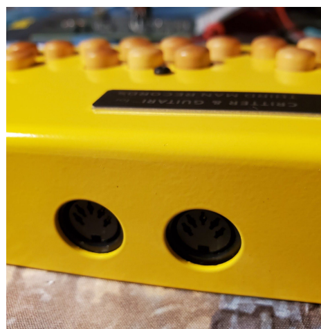
Fig. 1 The Critter and Guitari Septavox is an example of an instrument with MIDI in and out ports that can control other MIDI instruments or be controlled by a device such as the PAMC.
