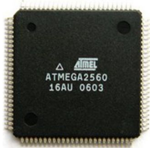
ATmega2560 QFP Package
