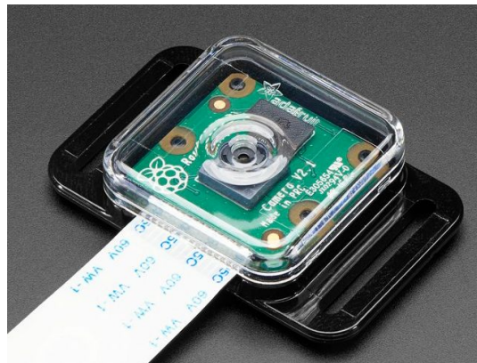
Figure 19: Waterproof casing for camera module
