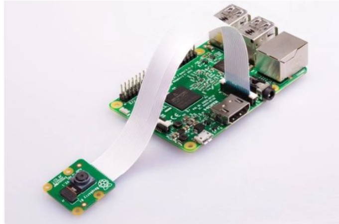
Figure #: Camera Module and Raspberry Pi Board connected through flex cable
