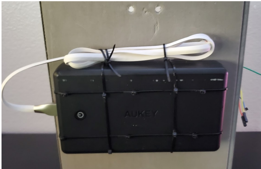
Figure 9.2.2: Portable battery mounted under base plate
