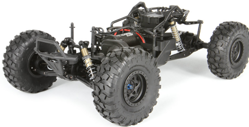
Figure 3.14.2: Independent Suspension on an RC Car (Reprint with permission-pending from AxialRacing)
