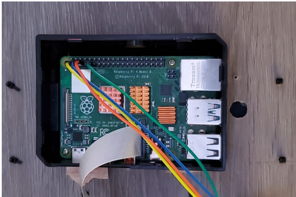
Figure 9.2.6: Raspberry Pi 4 mounted on base plate
