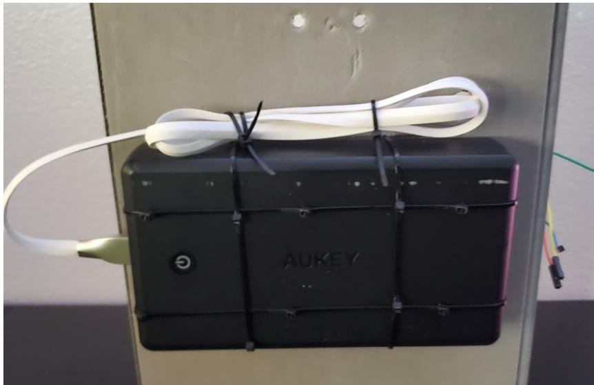
Figure 9.2.2: Portable battery mounted under base plate
