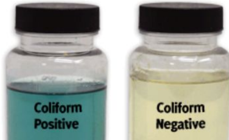
Figure 7: An example of two samples with a positive and negative result for coliforms
