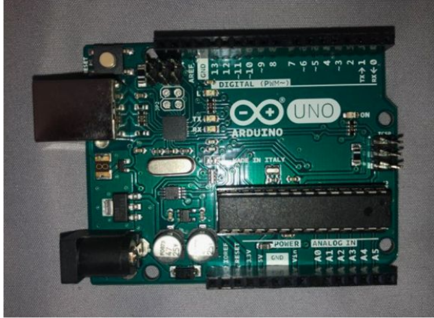
Figure 20: Arduino UNO board used for the PUVc analysis tank
