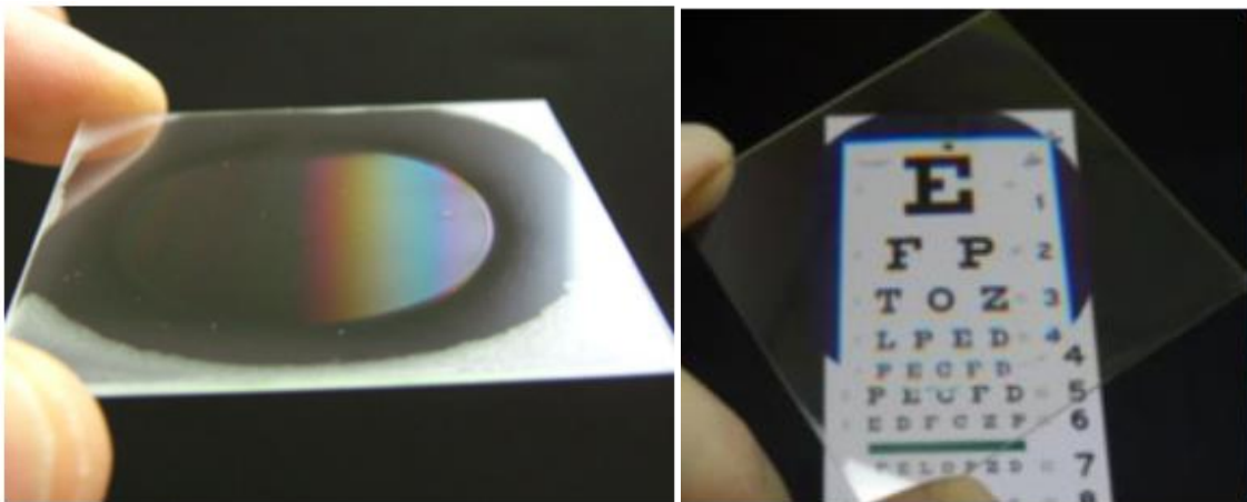
Figure 23 - Actual diffractive waveplate lens made from liquid crystal polymer, produced locally by BEAM Engineering Co. in Orlando, FL [51]
