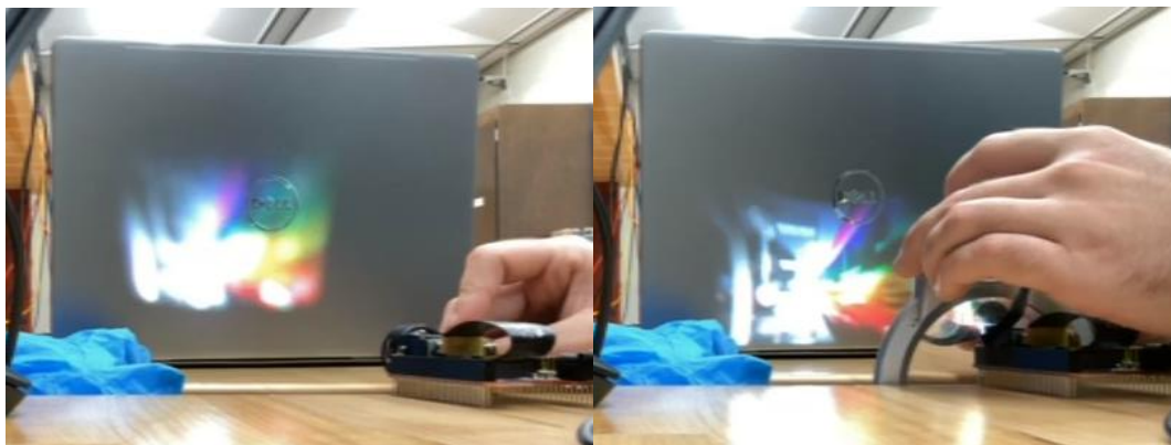
Figure 84 - Proof of concept that a two-lens system consisting of a positive lens followed by a negative lens would allow for magnification of the image, while keeping the image in focus
