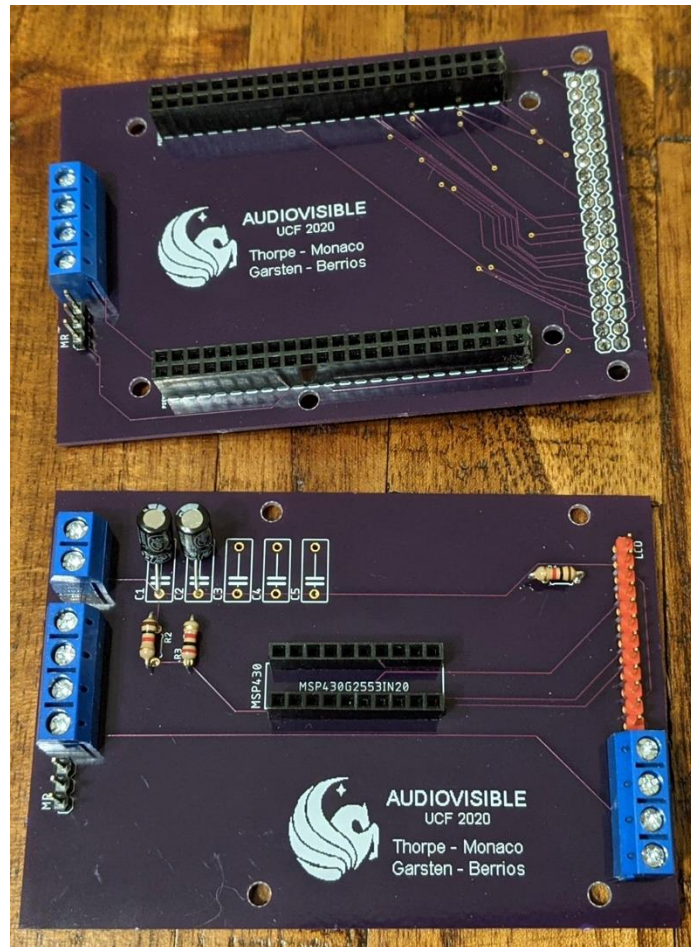
Figure 82 – PCBs after soldering components
