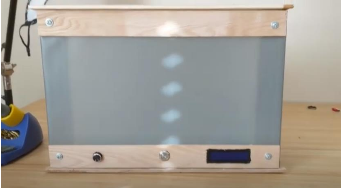
Figure 86 - Front panel of the AUDIOVISIBLE device. At the center is the viewing screen. Bottom left: Volume knob. Bottom Center: Power Button. Bottom Right: LCD status display
