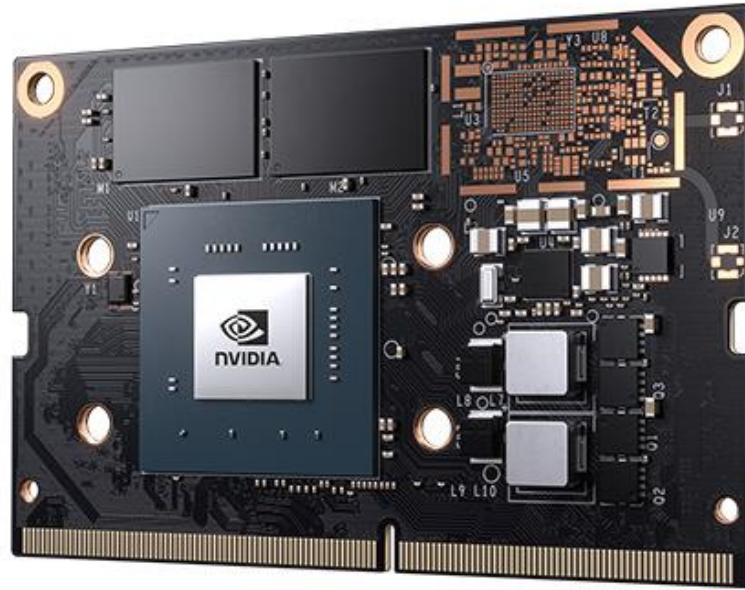
Figure 40 - NVIDIA Jetson Nano
