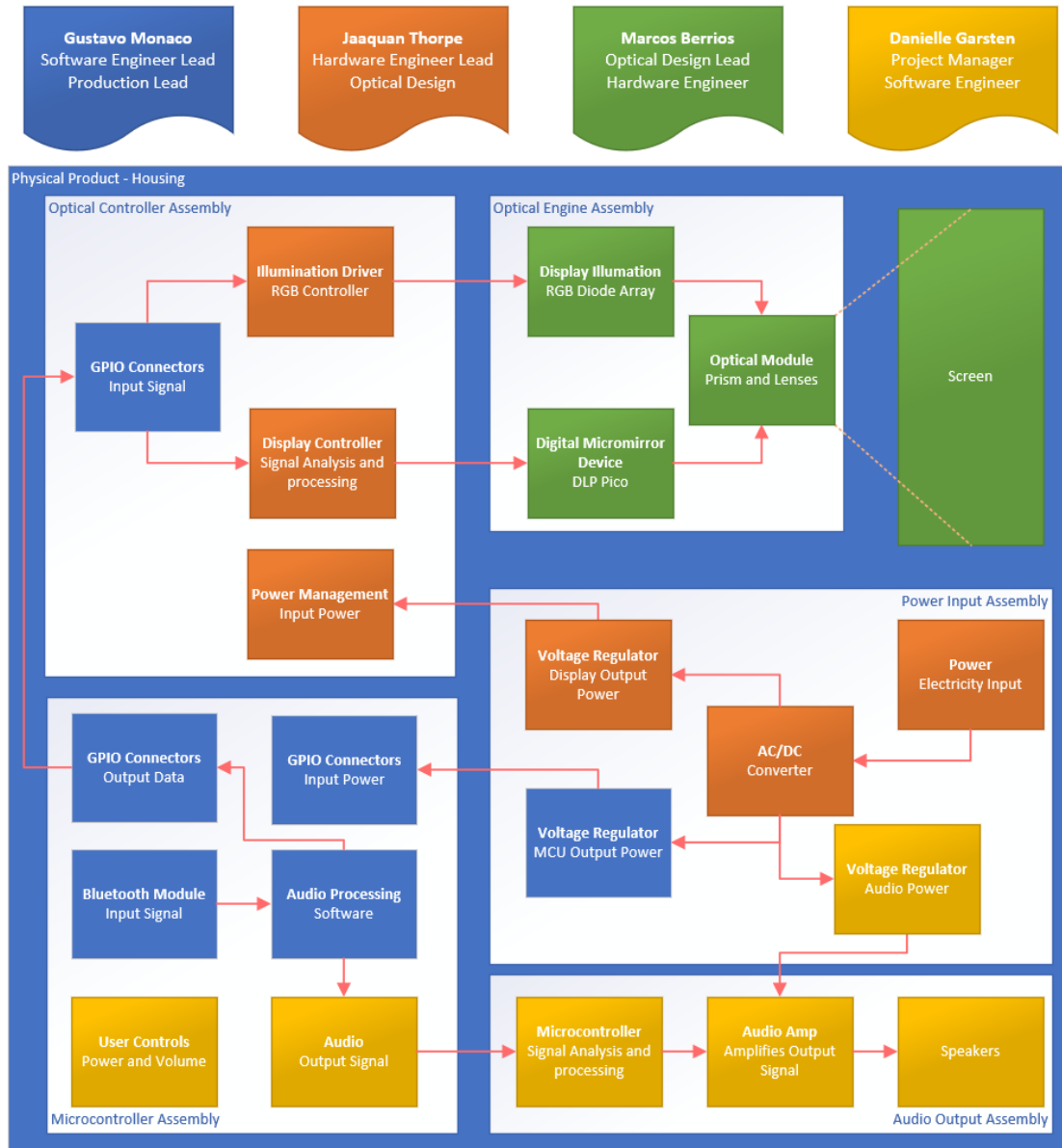
Figure 7– AUDIOVISIBLE System Block Diagram.
