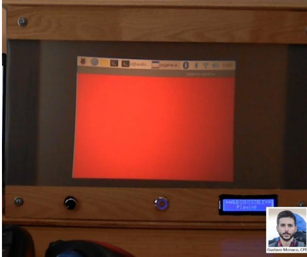
Figure 10 - Display of AUDIOVISIBLE device, visualizing the color red for a pitch with frequency of 375 Hz.
