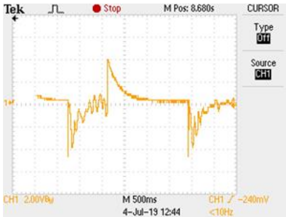
Figure 76. NIR Sensor AC Response at 3 Inches
