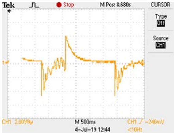
Figure 77. NIR Sensor AC Response at 3 Inches
