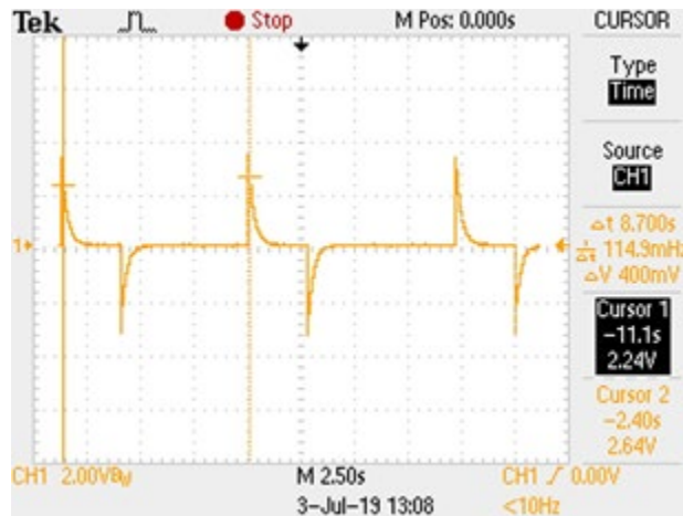
Figure 81. PIR Output for Consistent Triggering Measuring Period
