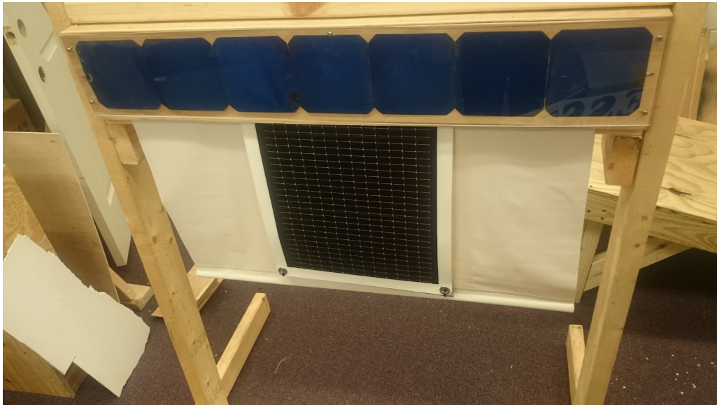
Figure 3.1.2.5 - 2015 'Solar Blinds' project window-facing side and wooden window frame.
