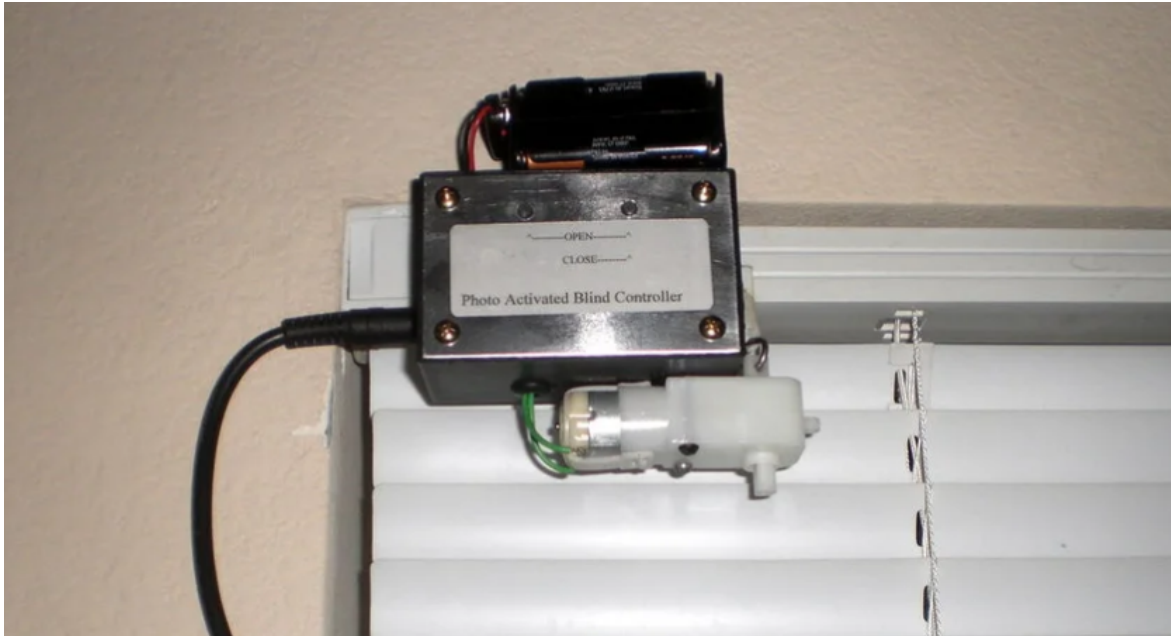
Figure 3.1.2.2 - Outward appearance for Biochemtronic's automatic blinds controller
