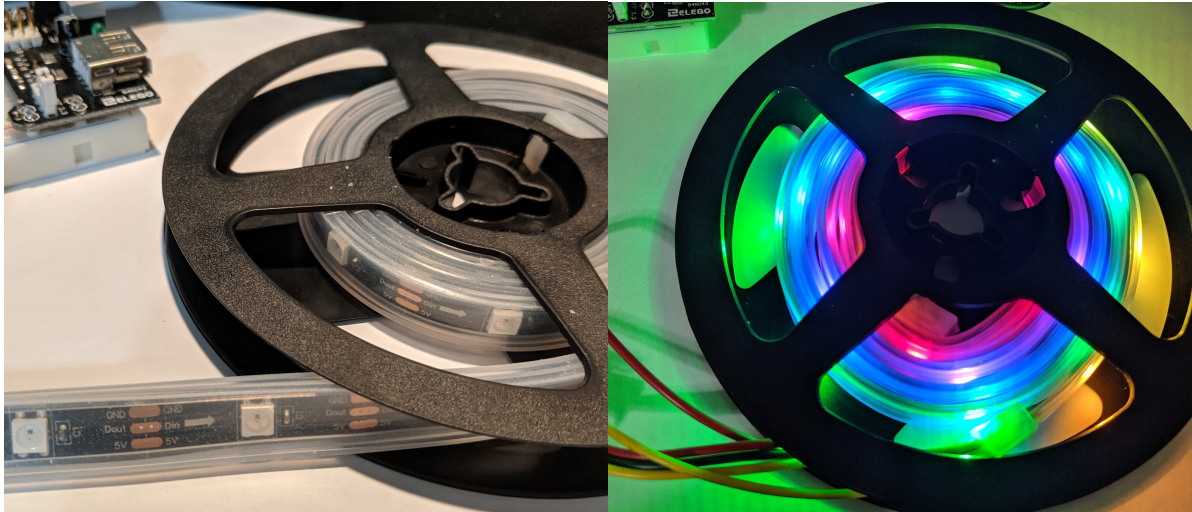
Figure 6.5.3.1 - (Left) Black 30 per meter NeoPixel strip with waterproof sleeve (Right) Strip during testing.
