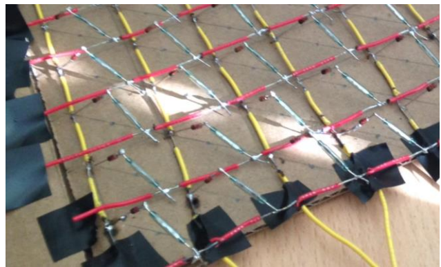
Fig. 6. Reed-switch matrix during construction
