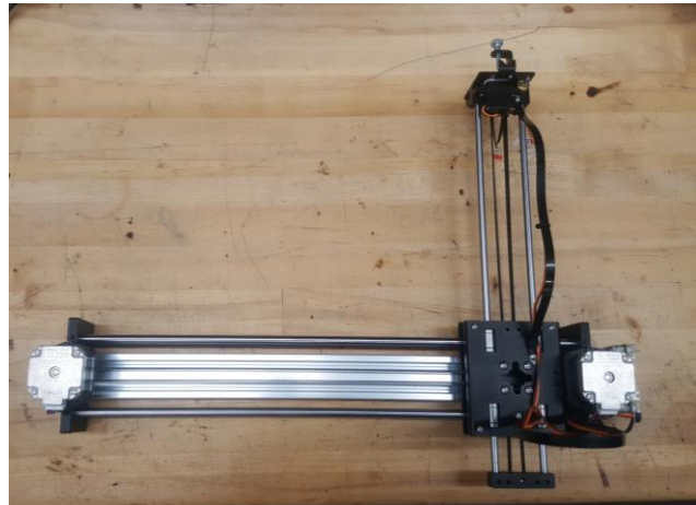
Fig. 2. IDRAW Machine XY plotter Physical presentation
