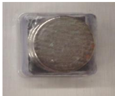
Fig. 3. A rounded neodymium magnet (18mm x 3mm) to place under the game piece
