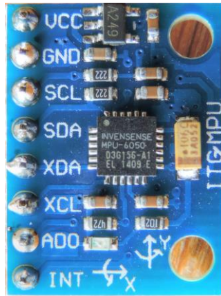
Figure 30 MPU 6050 Gyroscope and Accelerometer
