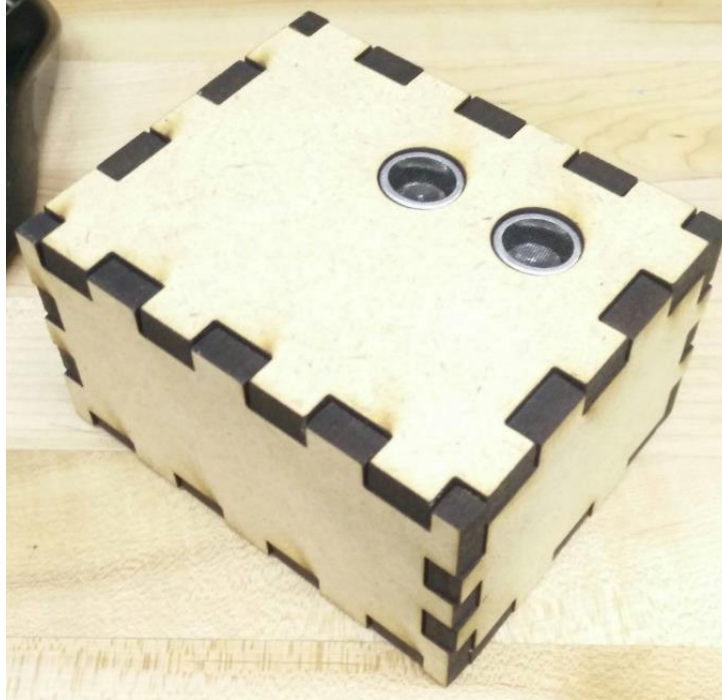
Figure 54: System housing for the sensor module.
