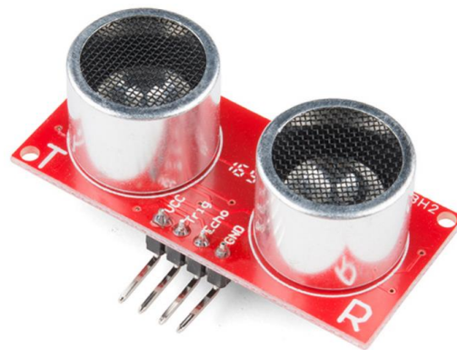
Figure 18: Ultrasonic sensor module. Reprinted with permission from SparkFun.
