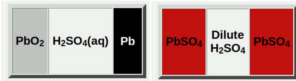
Figure 22: Lead-acid Battery Charged, Discharged (Left to Right) Permission Requested from: Battery University
