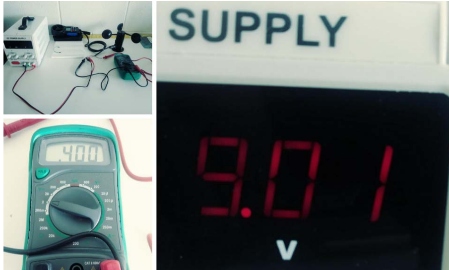
Figure 34 – Anemometer Voltage Test
