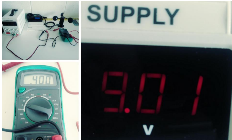
Figure 39 – Anemometer Voltage Test
