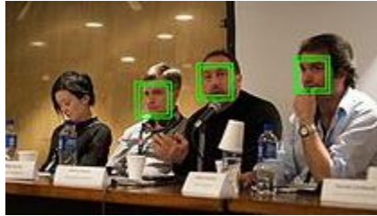
Figure 17 Automatic Face Detection with OpenCV
