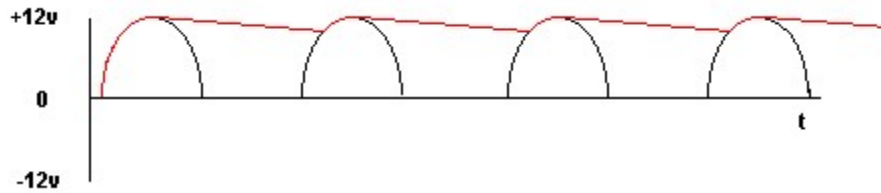
Figure 6 - Using a smooth capacitor on a half-wave rectified signal
