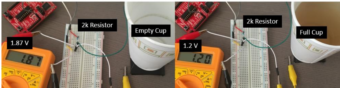
Figure 29: Weight Sensing Test with Velostat and Voltage Divider
