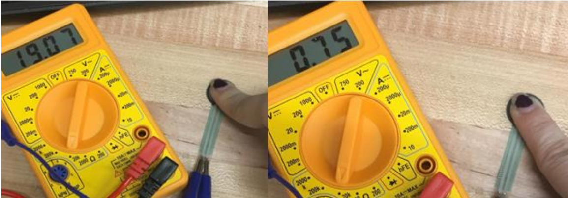
Figure 14: Reading resistance seen by the FSR. Light Pressing (left) and Hard Pressing (right)
