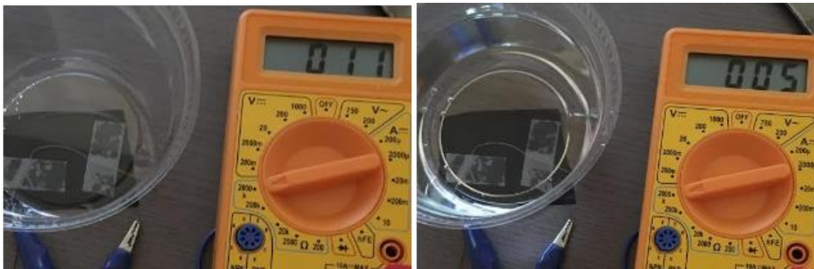
Figure 15: Empty Cup (left) and Full Cup (right) placed on top of piece of Velostat
