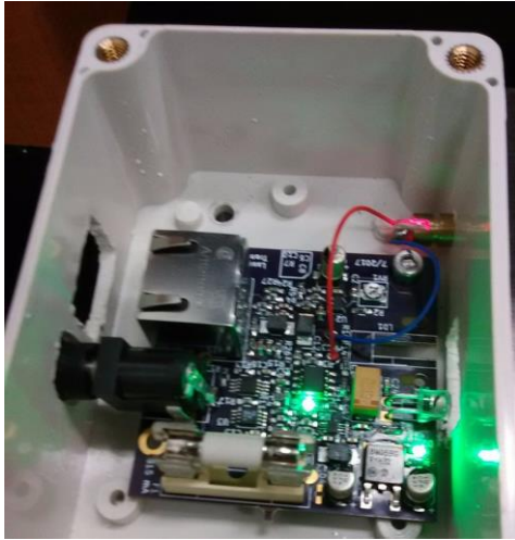
Figure 11. The final laser Ethernet transceiver design.
