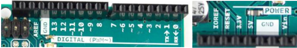
Figure 33: Digital PWN Pins (Left) and Power Pins (Right) on the Arduino Uno R3
