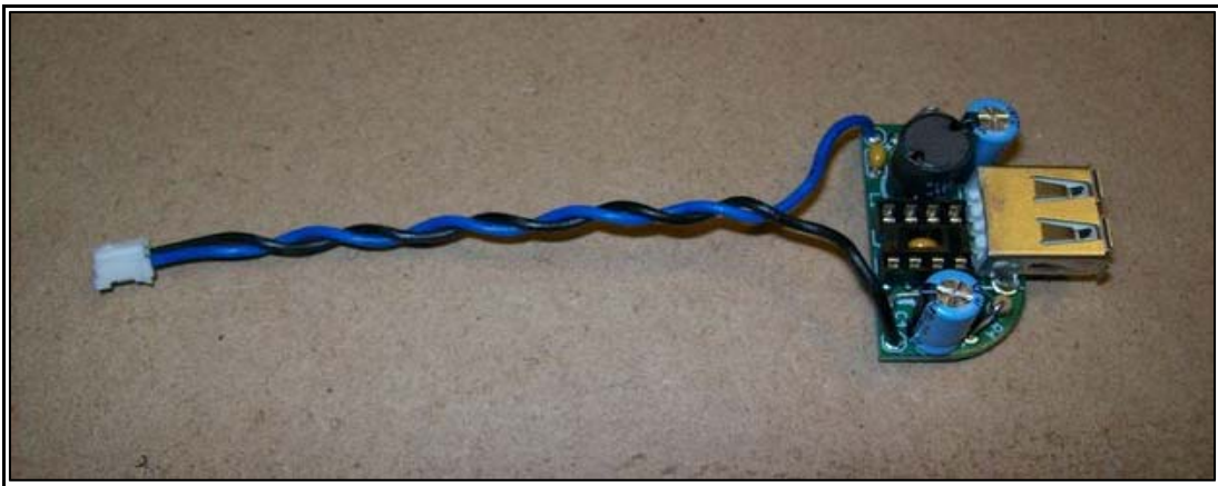
Figure 5 - MintyBoost Circuit with Added JST Connector
