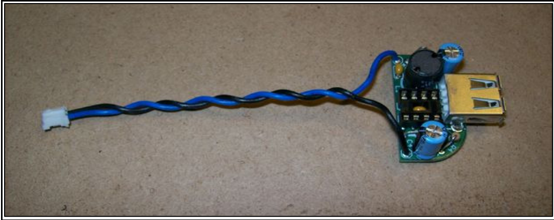
Figure 5 - MintyBoost Circuit with Added JST Connector
