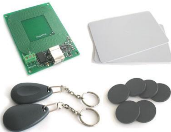
Figure 3-8 – Key card and keychain RFID tags. “Permission Pending”
