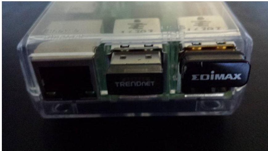
Figure 4.2.5 - Micro-Bluetooth and WiFi Adaptor
