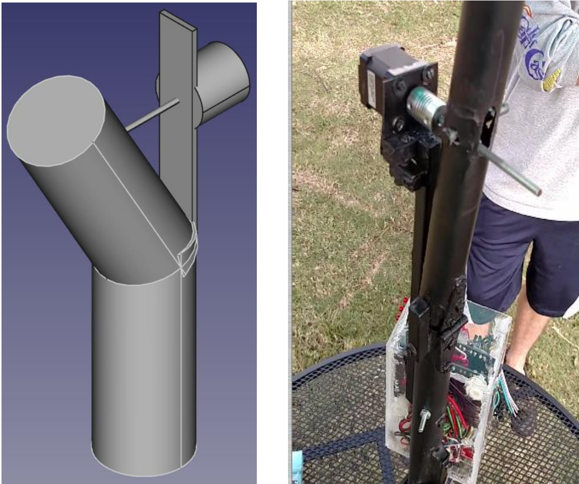
Figure 7.3-1 Original tilt motor model and final build of tilting motor
