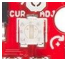
Figure 5.5-4 Current Potentiometer (Courtesy of Sparkfun Hook-up Guide)
